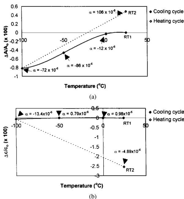
Figure 4 Percentage variation in the (a) basal plane area, (b) axial length for the cooling and heating cycles respectively. Values of  $\alpha$  (1/°C), calculated using adjacent data points, have also been included.
